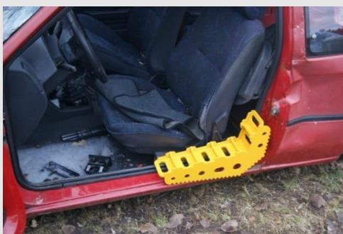
Support system for rescue rams designed to be used with all types and brands of tools available on the market. Perfectly adheres to the shape of spreading bodywork efficiently transferring the forces onto it. Provides safe and stable support in all necessary directions. Additional holes for belts or chains add up to versatility. Sturdy and durable made of 10 mm thick carbon steel. Suits modern vehicles.
