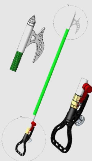
Innovative solution for fighting with internal fires. Combines pike pole hand tool with water mist lance to deliver water to areas with difficult access.
